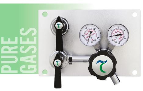
The LHPI 100P is a high purity gas supply panel. Manual adjustment of the regulator allow set a pressure. System include purge function. Designed for applications where a slight rise in delivery pressure from full to empty cylinder can be tolerated or as first stage of pressure reduction.
